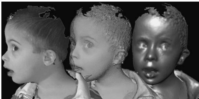
Fig. 1. Surfaces acquired by the 3dMD system. All surfaces were produced from the same image. Surfaces are shown at different orientations to illustrate 3D nature of the data. Left: smooth 3D geometry with texture map applied; middle: 3D wireframe geometry data (polygonal mesh surface); Right: smooth 3D geometry data.
